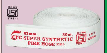
CRC Super Synthetic Fire Hose is made out of High Tenacity Synthetic Yarn to ensure fool proof performance The lining is seamless type of EPDM rubber compound for excellent protection against ageing and tackiness. The Synthetic jacket of the hose is completely inert against attacks from mildew and fungus. Moreover, being a 100% synthetic it can be dried very easily o form small and compact rolls which can stored and moved around easily.
